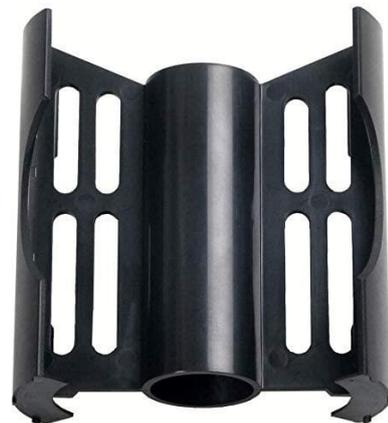
The idea is very simple. In the dark bag, you take your exposed 4x5 film sheet, flex it so that it curves and let it spring into place in the angles between two wings on one side of the reel. The reel is called a "spiral" for ease of description, but there's nothing spiral about it. It has two fins projecting from a central tube which fits over the tube in the Paterson tank. Each side can hold one piece of 4x5 film.
