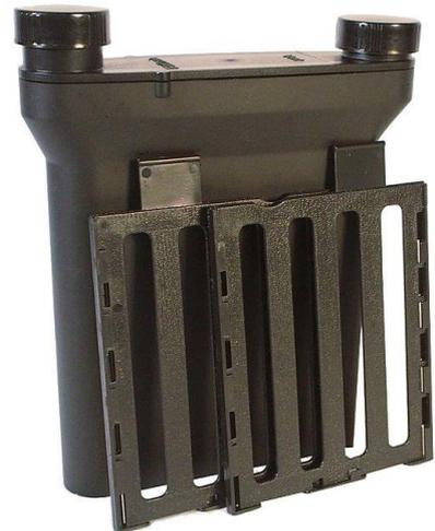
The tank is not much bigger than a 4x5 film sheet in area and about an inch thick. It's made light tight by a set of vertical baffles that have matching complementary cut-outs through which solutions flow. Between these baffles two film hangers slot in. The film sheets are held flat in these hangers by the edges in exactly the same way as in a dark slide, either side of the thin plastic film holder. There are two holders that slot between the baffles giving a capacity for four sheets in total.
